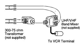
If your TV has both post and plug-type VHF terminals, the post connection is recommended to minimize signal loss.
